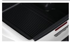
**UNDER RAIL BED LINER**Precision moulding for maximum load space, this polyethylene liner covers both the deck bed and side panels.
