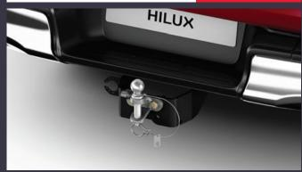
With its 3,200kg capacity, a Toyota towing hitch gives you plenty of load carrying flexibility.
